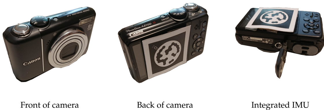
Figure 5.3: Digital camera with integrated IMU
